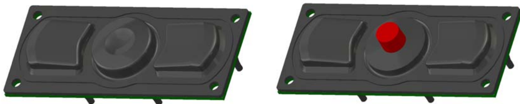
Figure 3: Exploded MicroModule Actuator Types (Left: Finger Disk, Right: MiniJoystick)
